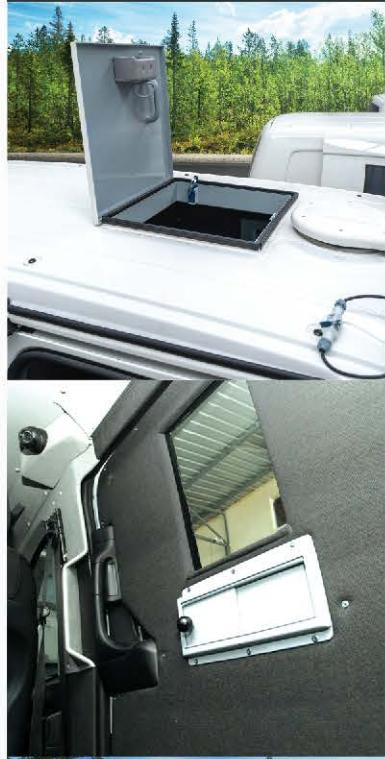
Vehicle Armoring is carried out at international standards at (BR2) - (BR6) levels and successfully passes all kinds of level tests, taking into account customer requests, the purpose of use of the vehicle, geographical threats, the licensed weapon allowed in the country and the presence of illegally used weapons. Armored Money Transfer Vehicles are designed and armored as Two Compartments, Three Compartments and Z Compartments.
