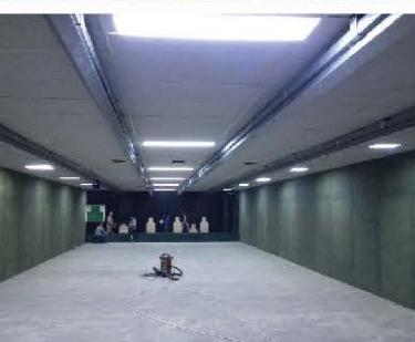
**Ground Coating:** The coating material to be used on the ground of the shooting polygon is made in a feature that does not bounce and swallow the bullet cores if the bullet core bounces on the shooting line for any reason and hits the ground.
